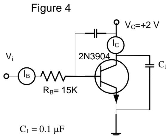
across the collector prevents oscillation that can be caused by the long leads going to the meter. The current gain,  $h_{fe}$ , depends on  $I_c$ . Specific examples can be seen in the specification sheets in the textbook.
